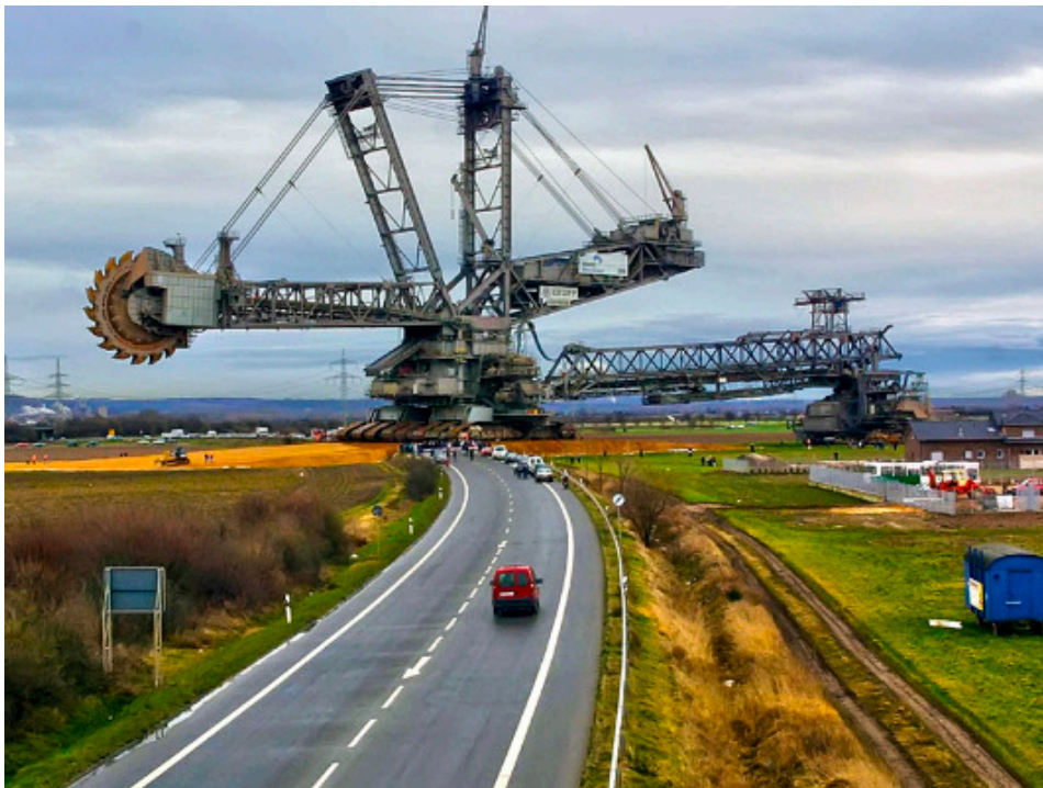
A self propelled MAN TAKRAF bucketwheel excavator (Bagger 293) crossing a road in Germany to get from one lignite mine to another. (Credit: u/loerez, Reddit)
