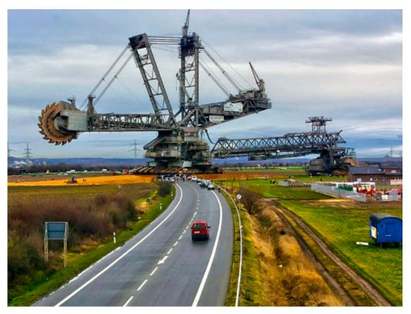
A self propelled MAN TAKRAF bucketwheel excavator (Bagger 293) crossing a road in Germany to get from one lignite mine to another. (Credit: u/loerez, Reddit)
