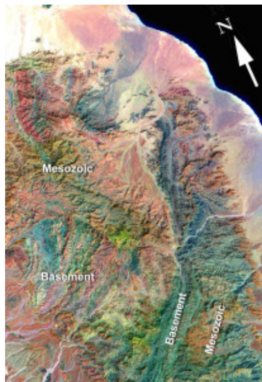
Geologically useful ASTER image of the Danakil Block in Eritrea/Ethiopia, showing Mesozoic and Recent sedimentary aquifers and crystalline basement (Steve Drury)
