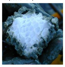
Gas hydrate (methane clathrate) block embedded in seabed
