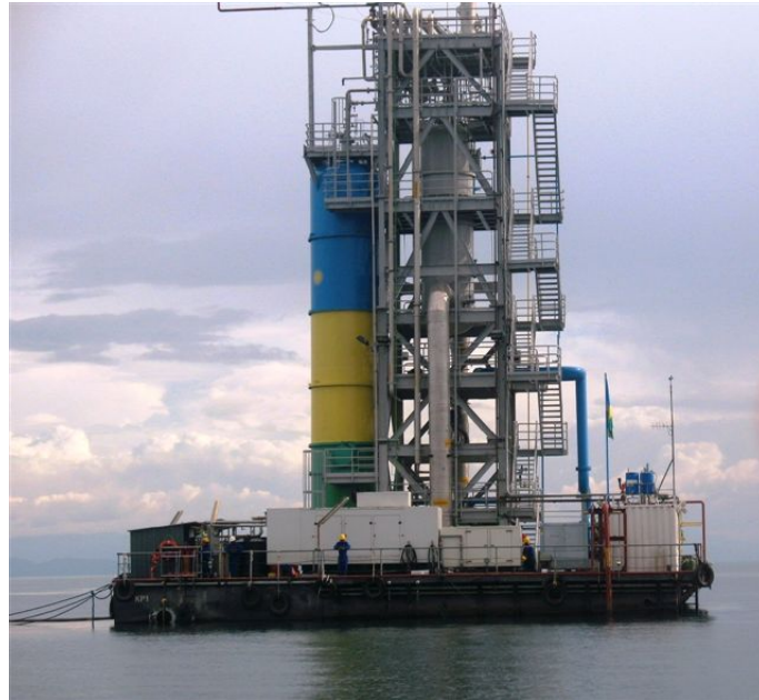
Methane extraction rig on Lake Kivu, DRC. (Credit: Wikipedia)
